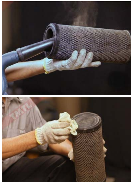
Cleaning of Air Cleaner element
