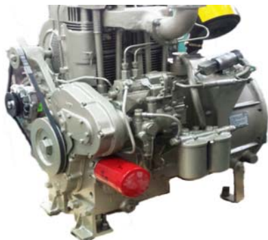
Oil Filter Replacment 323 ES
