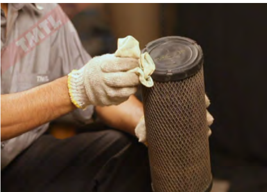
Cleaning of Air Cleaner element
