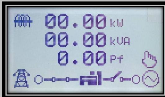
Combined Active Power, Apparent Power & Avg. Power Factor
